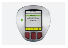
Built-in data recording capability allows the user to maintain a log of all completed bolting jobs. For improved quality control and accountability, the information can be saved to a PC or tablet to provide a permanent record of the work performed.
